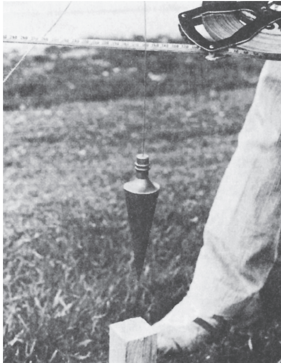
FIGURE 1.5 Preparing to measure to a stake tack, using a plumb bob and steel tape.
